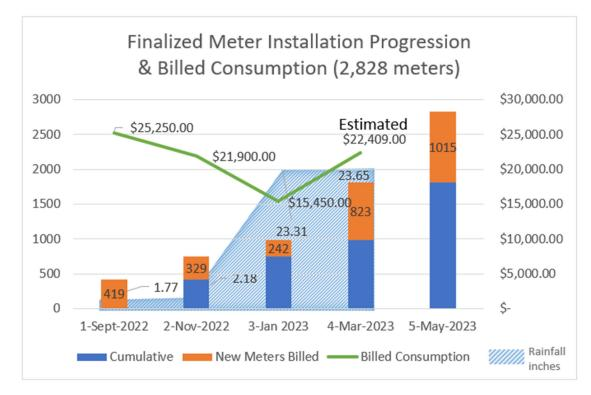
Finalized meter installations are meters which are fully reporting for 30 days with reading data available to billing staff through our meter reading portal.
