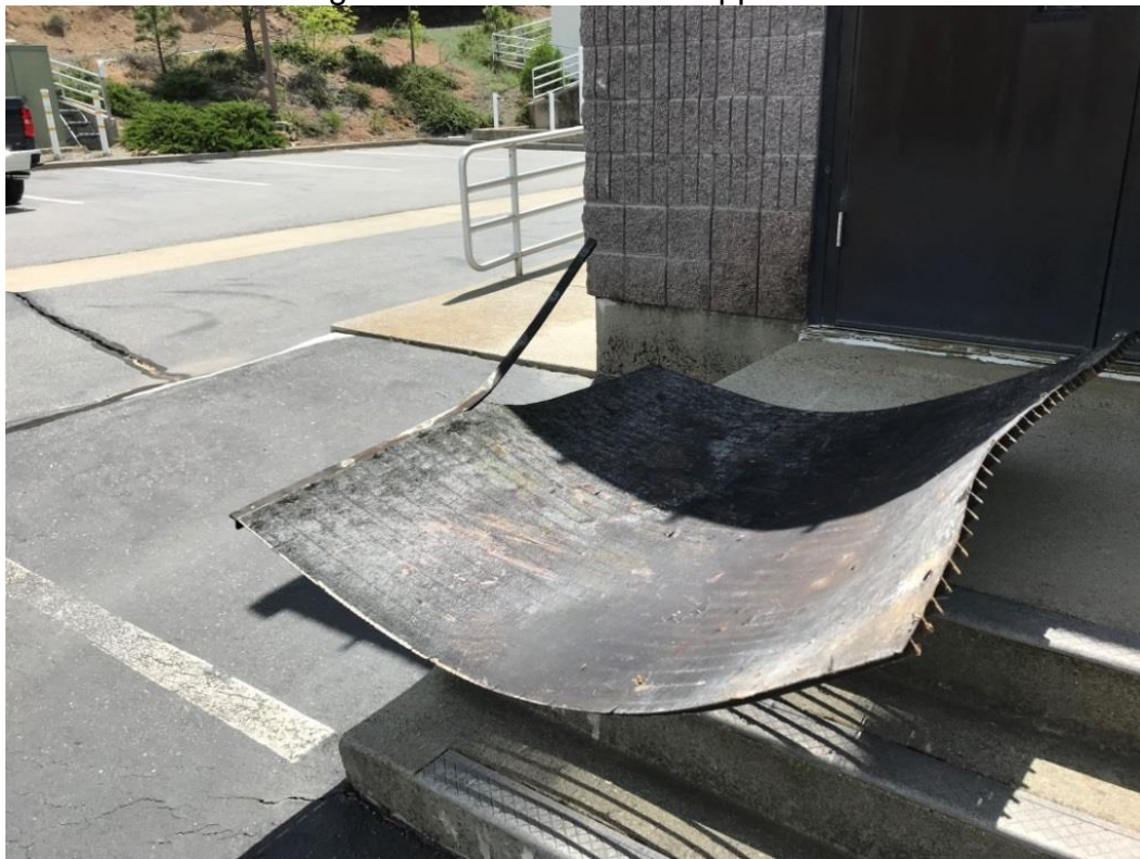
The Damaged Screen Section is Supposed to be Flat
